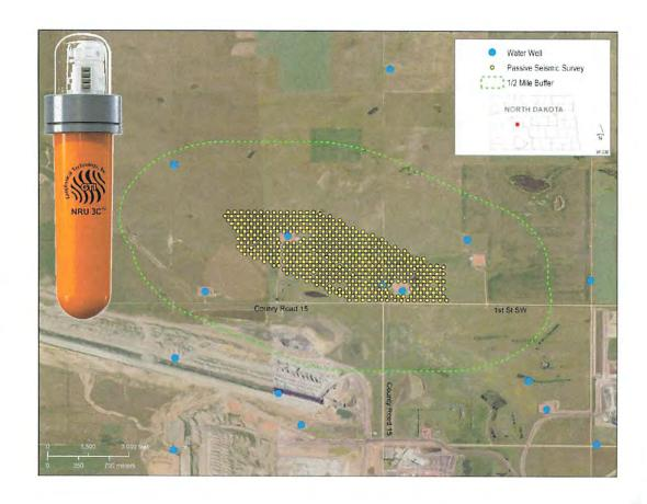
Map of passive seismic sensor deployment. Sensors will be buried 3-5" in a regular spacing along the thin blue lines.
